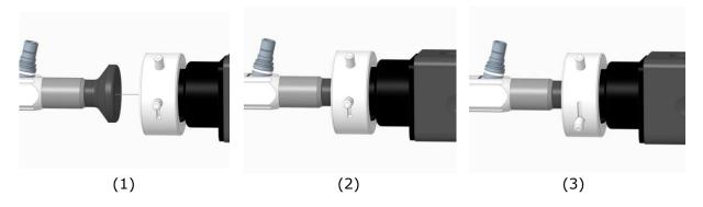
• Unlock the camera head (1) as shown in the picture and put it on the eyepiece funnel (2) and lock it (3). Due to the different compatible systems, the instructions for use from the manufacturer must be followed.
