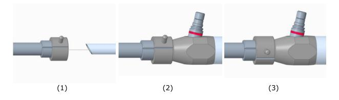
• Unlocking the camera head (1), placing it on the eyepiece funnel (2) and locking the camera head (3). as shown in the picture. Due to the different systems, the instructions for use from the instrument manufacturer must be followed.
